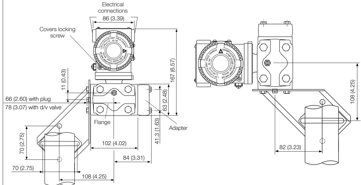
NOTE : Process connection, gasket groove and gaskets are in accordance with DIN 19213. Bolting threads for fixing adapter or other devices (i.e. manifold etc.) on process flange is  $7/16$  – 20 UNF.
