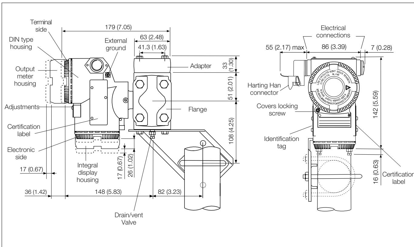
**Transmitter with barrel AISI ss housing on bracket (flat type for box) for vertical or horizontal 60mm (2in) pipe mounting**
