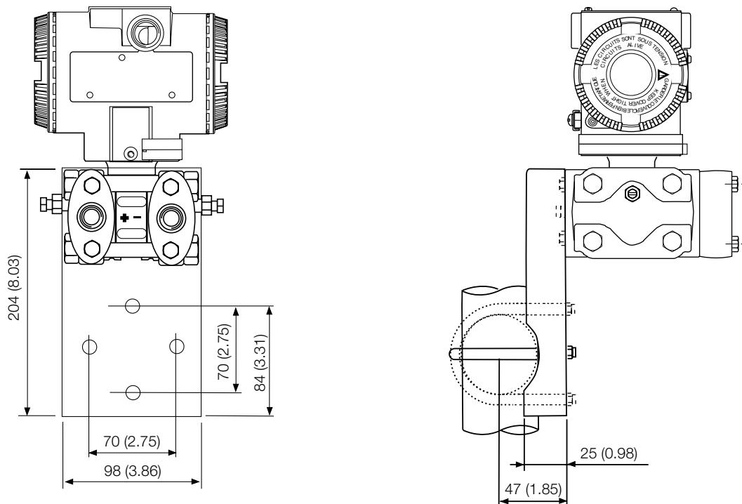
**Transmitter on bracket for wall mounting (by up to four M8 screws, NOT SUPPLIED)**
