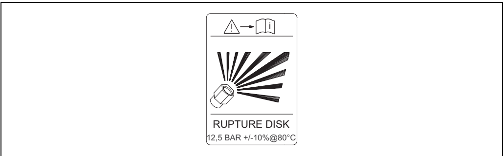
Indication label for the rupture disk
