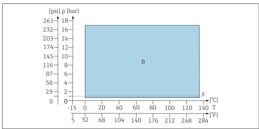
图 5 Pressure/temperature ratings
