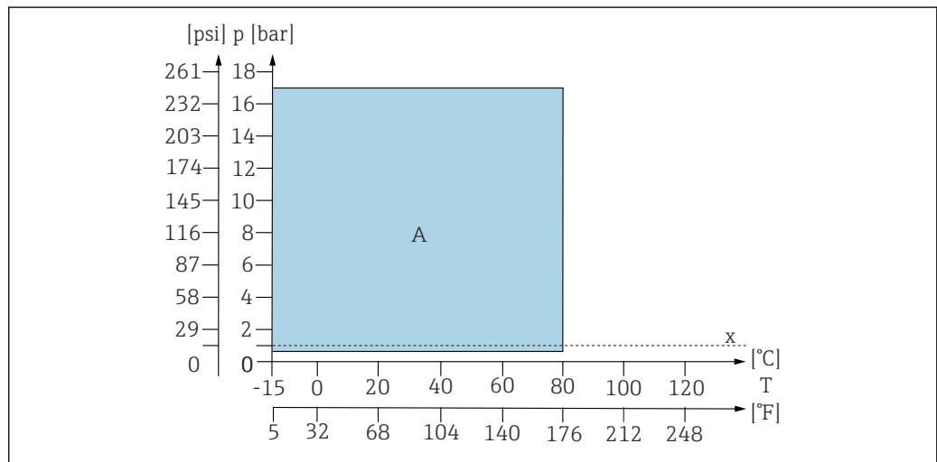
图 4 Pressure/temperature ratings
