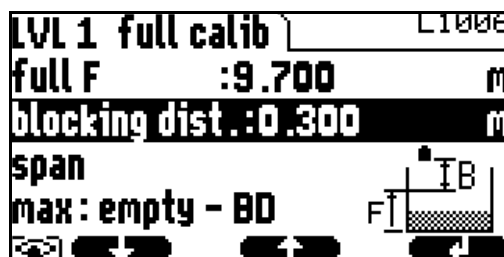
Display of a function including help text and descriptive graphic
