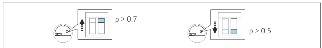
56 Switch position on the electronic insert for density
