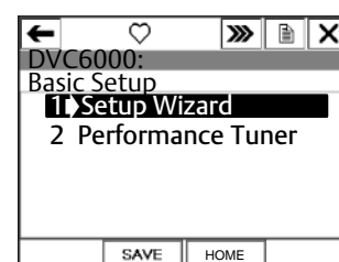
Figure 19. Accessing the Setup Wizard on the Field Communicator (Instrument Level HC, AD, and PD)
