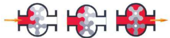
Figure 2, Bi-rotors inner measuring chamber.
