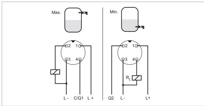
Wiring plan (housing), terminal assignment IO-link output with M12 x 1 plug connection
