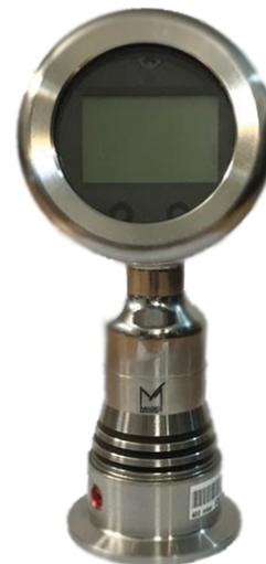
The measuring range covers 0 ... 250 mbar up to 0 ... 200 bar. The MDS6 pressure transmitter is powered with a DC voltage of 10 (14) ... 30 V. Available electronic output signals are 4 ... 20 mA, 0 ... 20 mA or 0 ... 10 V output.
