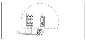
Fig. 13: Connection HART two-wire, Profibus PA, Foundation Fieldbus
