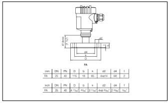
Fig. 24: VEGABAR, flange connection form B1, EN 1092-1
