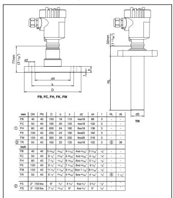
Fig. 32: VEGABAR 65, flange fitting
