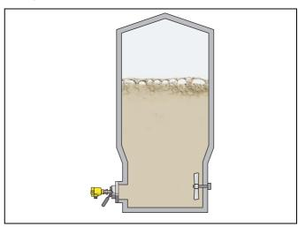
Fig. 6: Level measurement on storage towers with VEGABAR 54
