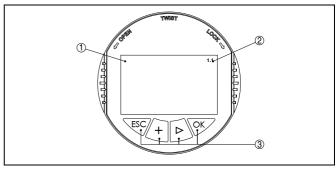
Fig. 16: Indicating and adjustment elements
