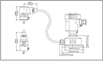
Fig. 22: Transmitter and remote housing with IP 68 version
