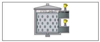
Fig. 7: Pressure measurement on a screen with VEGABAR 54
