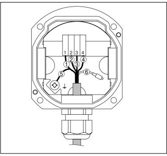
Fig. 15: Connection of the sensor in the housing socket
