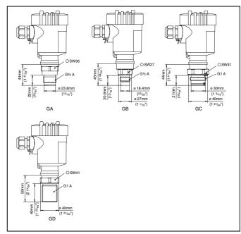
Fig. 23: VEGABAR 55, threaded fitting
