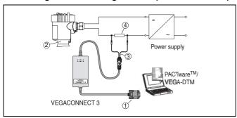
Fig. 18: Connecting the PC to the signal cable
