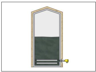
Fig. 10: Level measurement in a bitumen vessel with VEGABAR 65
