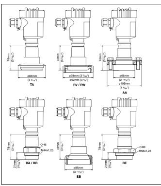
Fig. 31: VEGABAR 65, threaded and hygienic fitting - part 2
