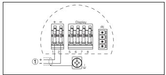
Fig. 12: Connection HART two-wire, Profibus PA, Foundation Fieldbus
