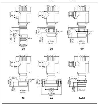
Fig. 26: VEGABAR 64, threaded and aseptic fitting
