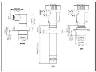
Fig. 30: VEGABAR, extension fitting for paper industry
