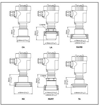
Fig. 27: VEGABAR 64, threaded and aseptic fitting
