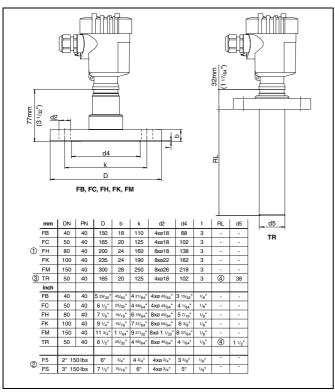
Fig. 33: VEGABAR 65, flange fitting
