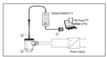
Fig. 17: PC connected directly to the sensor
