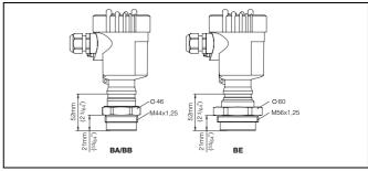
Fig. 29: VEGABAR 64, threaded fitting for paper industry
