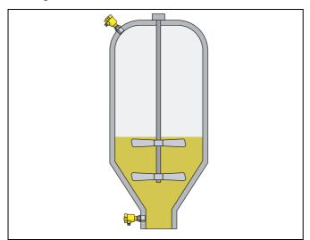
Fig. 9: Level and pressure measurement in a feeding vessel in the ointment production with VEGABAR 65
