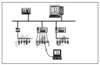
Fig. 11: Integration of instruments in a Profibus PA system via segment coupler DP/ PA or data recording systems with Profibus PA input card
