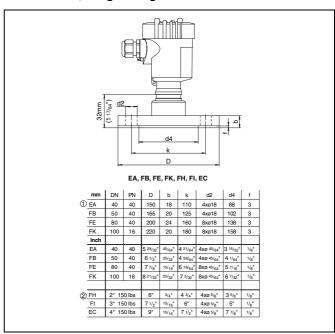
Fig. 28: VEGABAR, flange connection
