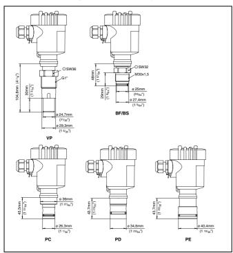
Fig. 25: VEGABAR 54, fitting for paper industry
