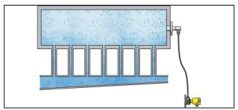
Fig. 8: Pressure measurement on the headbox of a paper machine with VEGABAR 64
