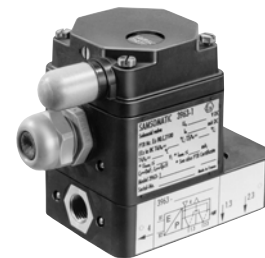
5/2-way solenoid valve, single actuated with spring return mechanism, K_{vs} 0.16, connection G 1/4
