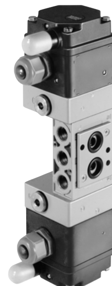
5/2-way solenoid valve, double actuated with two locking positions, K_{vs} 1.4, connection G 1/4 /NAMUR
