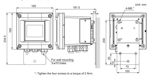
Note: For wall mounting, the wall should be strong enough to bear the weight of 8 kg or more.
