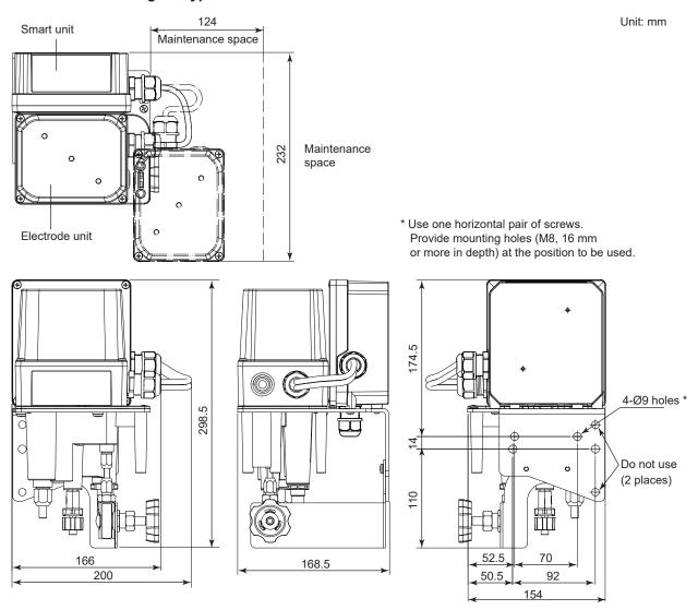
Note: For wall mounting, the wall should be strong enough to bear the weight of 15 kg or more.
