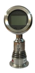
The measuring range covers 0  $\dots$  250 mbar up to 0  $\dots$  200 bar. The MDS6 pressure transmitter is powered with a DC voltage of 10 (14)  $\dots$  30 V. Available electronic output signals are 4  $\dots$  20 mA, 0  $\dots$  20 mA or 0  $\dots$  10 V output.
