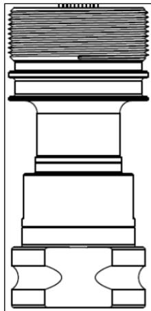
Figure 32 – Inline Gauge and Inline Atmospheric Meter Body Bodies
