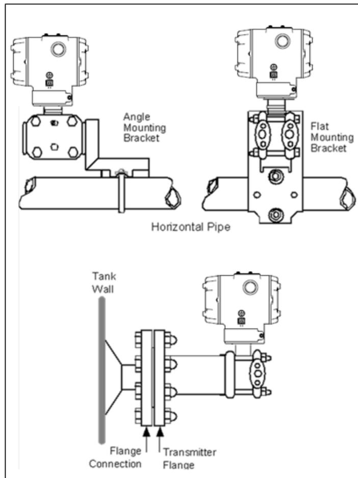
Figure 4 – Typical Bracket Mounted and Flange Mounted Installations
