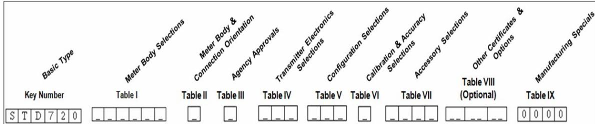
Figure 3 –Typical ST 700 Name Plate
