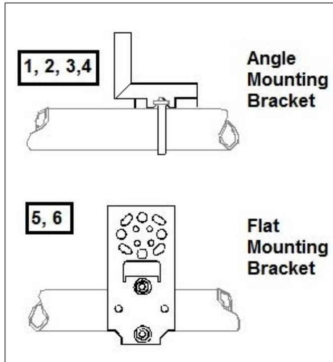
Figure 26 – Angle and Flat Bracket Parts
