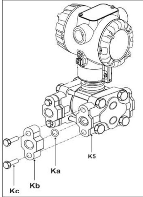
**Figure 12 – Flange Adapter Removal and Replacement**
