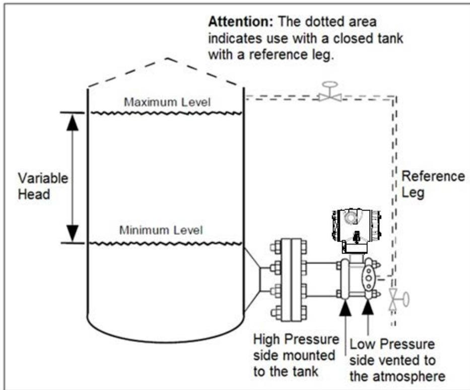
Figure 9 – Tank-Flange Mounted Transmitter
