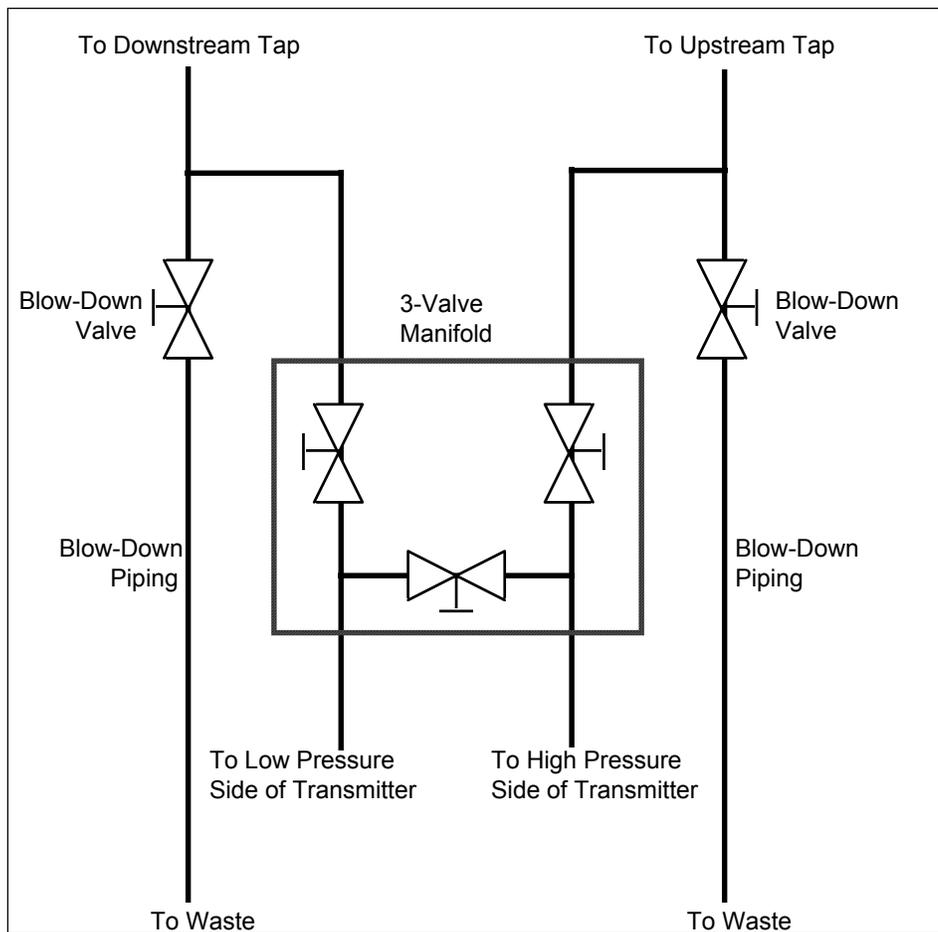
Figure 11 – Typical 3-Valve Manifold with Blow-Down Piping
