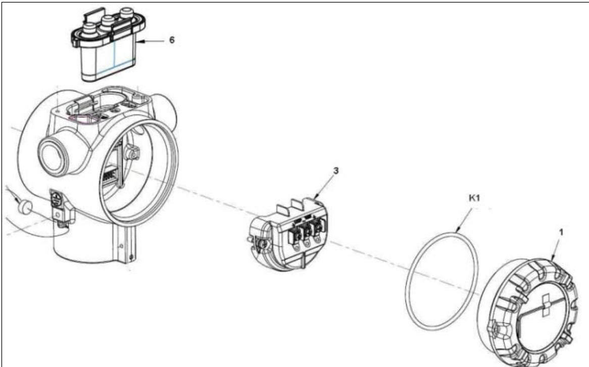
**Figure 28 – Electronic Housing, Terminal Block End**
