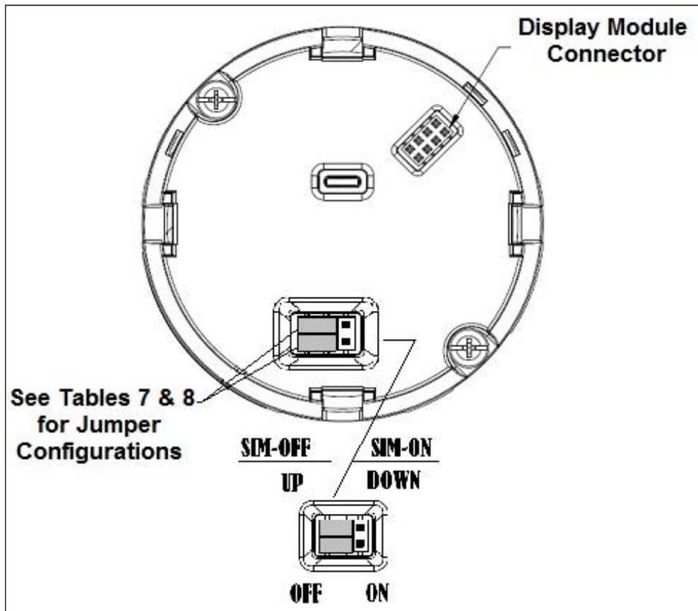
Figure 17 – Locating the Failsafe and Write Protect Jumpers
