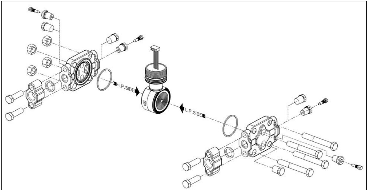
Figure 31 – STG730, 740, 770, and STA722, 740 Transmitter Body (Ref.)
