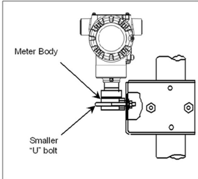
**Figure 6 – In-line Model Mounted to an Optional Bracket**
